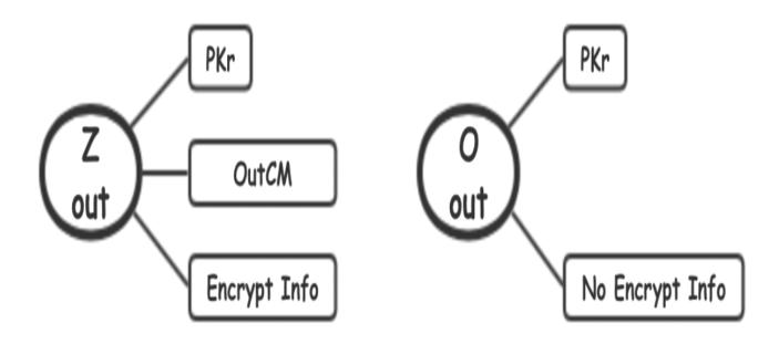
The outputs contained in HCT transactions are divided into two forms, zero-knowledge output Z out and ordinary output O out.
